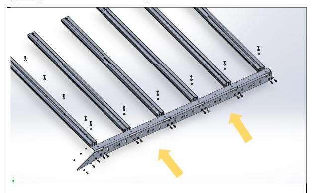
1. Fit the side rail to the extrusions,
